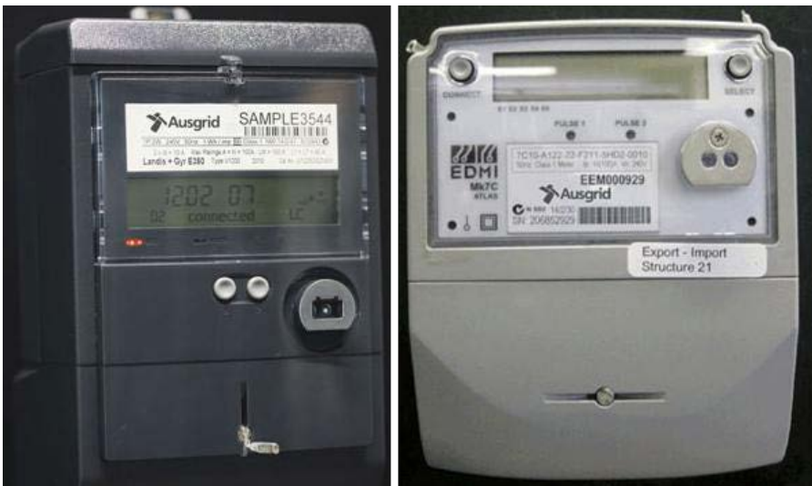
Smart meter and interval meter
